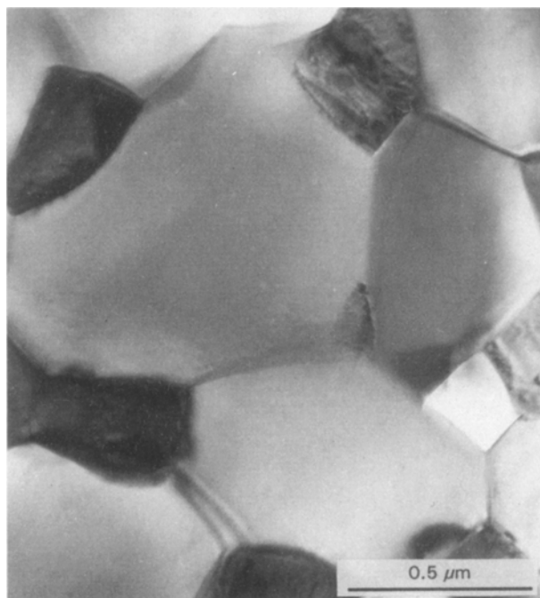
Figure 2 Transmission electron micrograph of as-sintered sample at 1450^\circ\text{C} in Y-ZTA.
